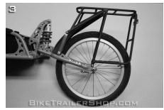
**nut**. If you don't, the bolt will loosen, and the trailer eyelet threads could be damaged when the rack is under load. Double-check all your fasteners, (especially the 30mm bolts at the trailer dropout eyelets!).
