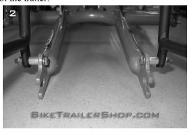
2. Attaching the Greenspeed rack to the dropout eyelets on the trailer
