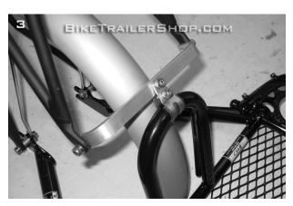
3. Attaching the adapter bracket to the upper rack eyelets Align the holes in the upper rack eyelets with the adapter bracket. Put a M5 x 10mm washer on a M5 x 12 mm bolt, slide it through the rack eyelet, and thread it into the adapter bracket. Repeat this process on the other side
