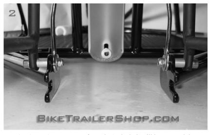
that you hold it in place with an allen key while tightening the nut. If you don't, the bolt will loosen, and the trailer eyelet threads could be damaged when the rack is under load.
