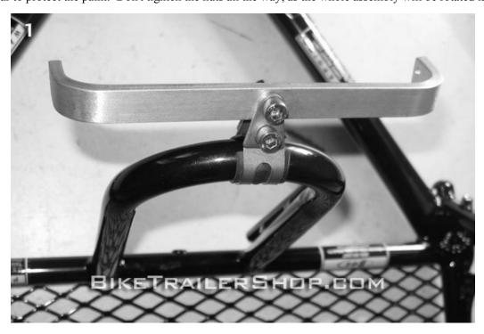
2. Attaching the Greenspeed rack to the trailer dropout eyelets
